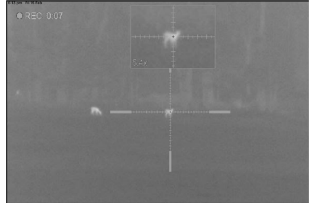
Figure 7. Use of Thermal Imagery to detect deer activity in low light
